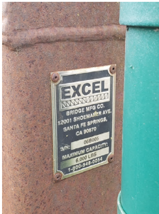
Image 12: Bridge Capacity Plaque
